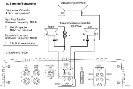
\*You may change the subwoofer satelite crossover frequency by using the Inductor and Capacitor values calculated with the following formulas: High Pass (Satelite Crossover): 30,000 Design descent particular = New Capacitor Value in μF
